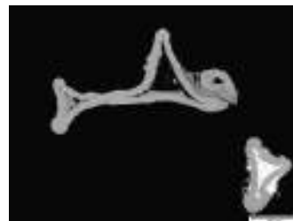
Detail illustrating partial filling of the copper struts by the solder alloy
